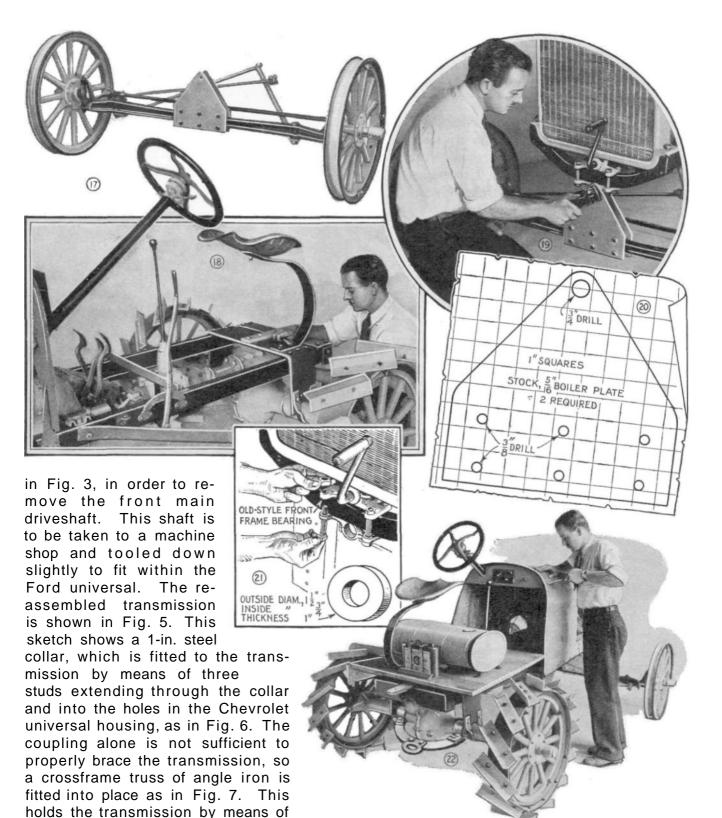
two long bolts, properly spaced by means of two 1/2-in pipe nipples. A second trip to the machine shop is necessary to have the shaft splined as shown in Fig. 8. The heavy portion is already splined to fit the Ford truck differential of which it is a part, but the splines on the lower half must be machined to fit the Chevrolet universal, as shown in Fig. 12. Next, a 5-5/8-in. length, cut from the rear of the Ford truck driveshaft housing, is brazed
